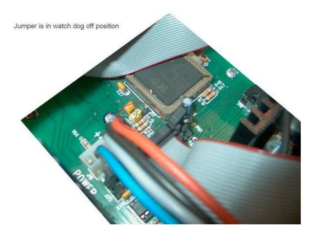
There are some regulations that advise to use a watchdog for safety. In case of software-malfunction (freeze) the watchdog will force a reset of the CPU.
